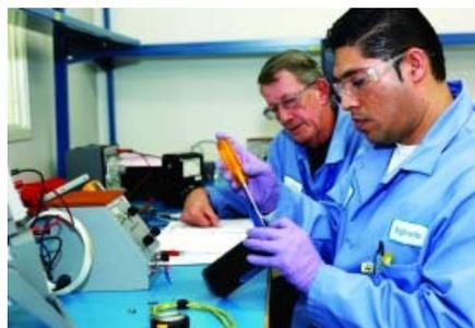
Working on capacitance probes on the fuel quantity indicating system for the Airbus A320 are Ontic's electronics lead Pedro Paiva and electronic technician Sigfredo Mendoza.
