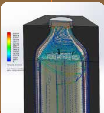
Hydrogen flow velocities at the upper end of a Centrifugal Fuel Element of the CNTR. Image Courtesy: SolidWorks plot, Zack Sakata, Center for Space Nuclear Research.
