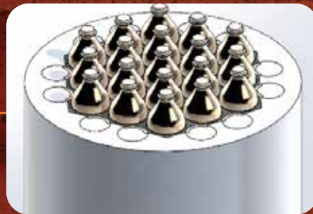
Top view of the CNTR showing the upper (turbine) ends of the 19 Centrifugal Fuel Elements surrounded by the 12 control drums. Image Courtesy: Zach Sakata, Center for Space Nuclear Research.
