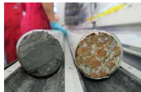
Rock cores recovered from the Chicxulub impact crater. Image courtesy: MARUM/MMowat@ECORD/IODP
