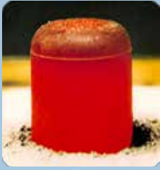
Pellet of ^{238}\text{PuO}_2 , glowing due to decay. Image courtesy: NASA
