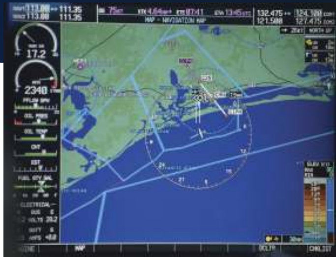
The Multi Function Display in the CAP Cessna 182 shows traffic inside the restricted area.
