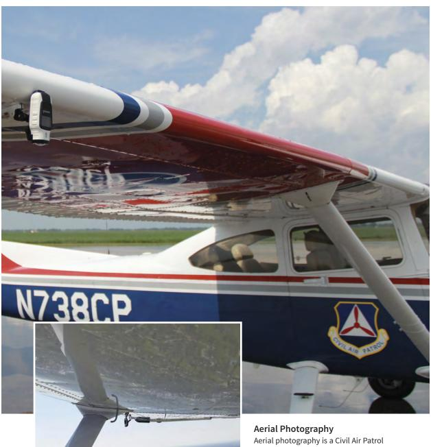
Aerial photography is a Civil Air Patrol core mission, one made easier with state-of-the-art Garmin VIRB cameras attached to the wings of CAP planes, allowing for ground images from directly above. These wing-mounted cameras were used to assess damage in the wake of Hurricane Matthew flooding in 2016.
