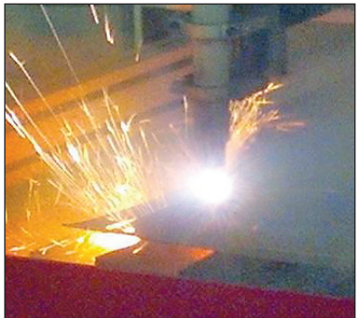
PLASMA — The plasma cutter in action sends up a brilliant display of sparks as it cuts metal. Pella Corporation’s acquisition of Weather Shield in July and during Manufacturing Month this October,
