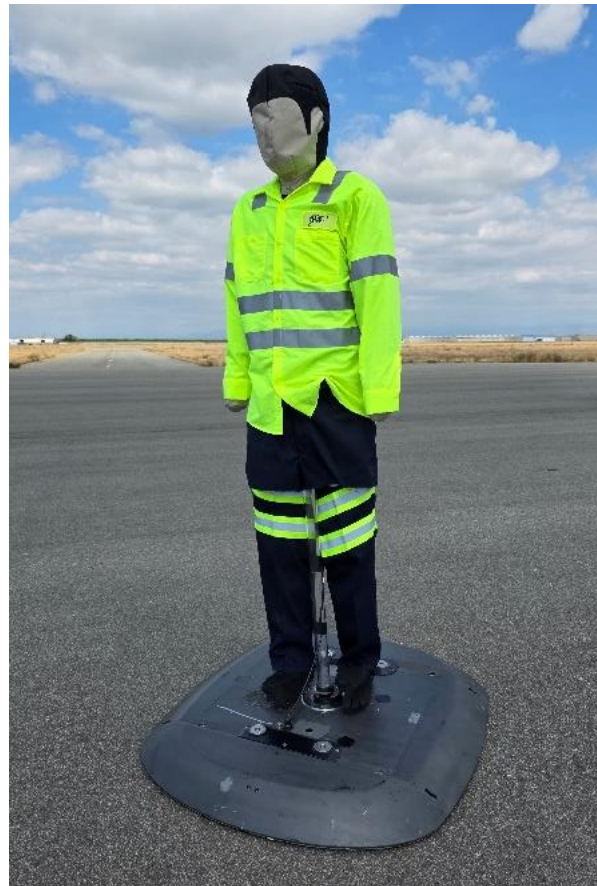
Figure 10: ABD LP80™ with 4activePA-adult Articulating Pedestrian Target in ANSI Class 3 Attire.
