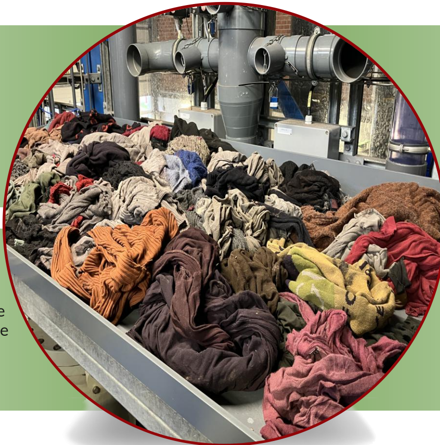
Polyester residue of postconsumer polycotton waste textiles in the DAWN pilot plant
